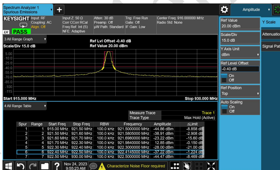
图 4-2.17 922M 125K Radio channel Spurious Emission
