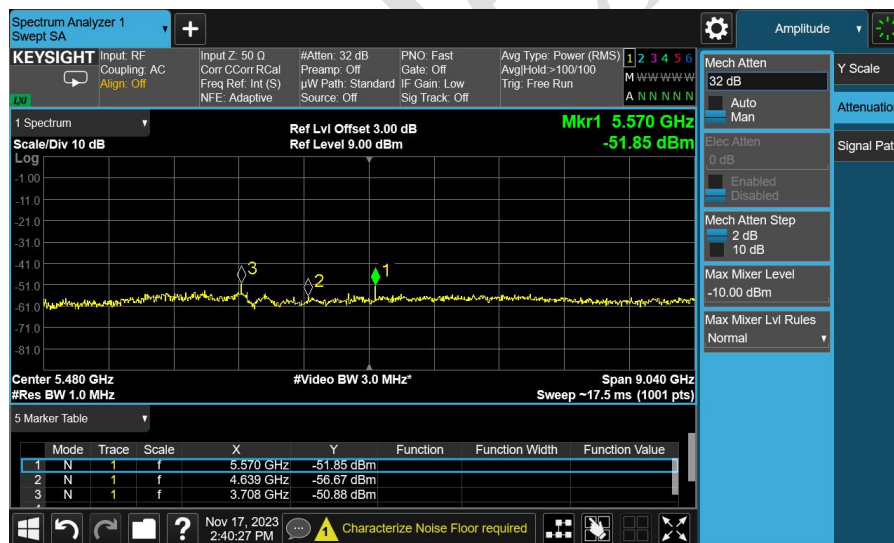
图 3-1.15 TX:928M 500K TEST BAND:Above 960M RF Antenna Conducted Spurious Emission
