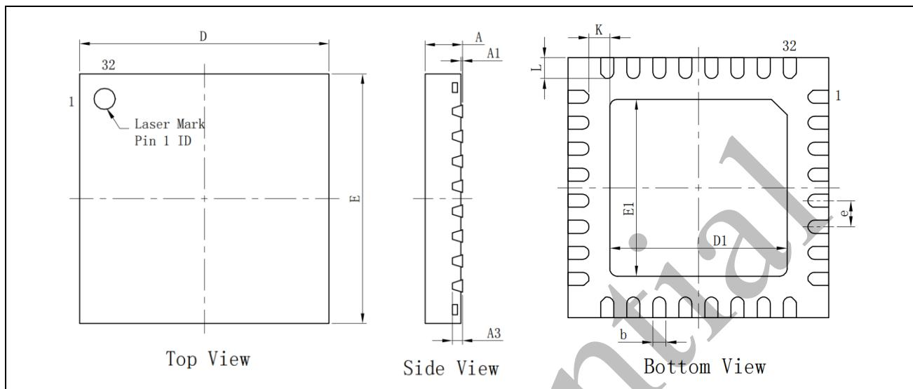
Figure 7-1 QFN32(5×5) package view
