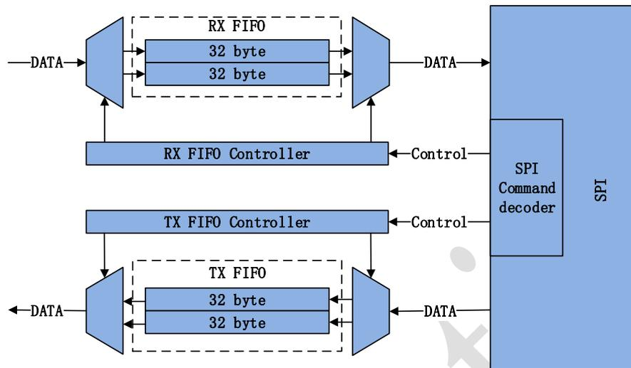
Figure 5-4 FIFO diagram
