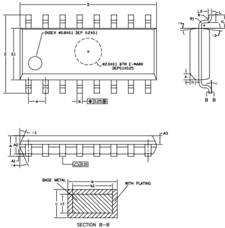
Figure 10-3 XN297L SOP16 package
