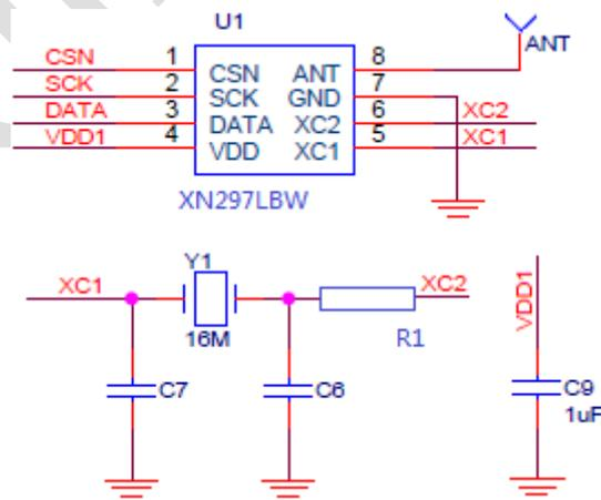
Figure 9-2 The XN297L schematic for package of SOP8
