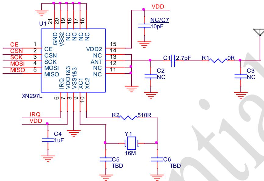
Figure 9-1 The XN297L schematic for package of QFN20 3\*3
